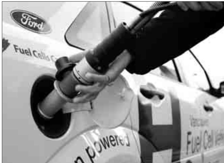
CLOCKWISE FROM TOP LEFT: BC Hydro's Ford Focus fuel cell vehicle (one of five in the Vancouver Fuel Cell Vehicle Program) beside the Hydrogen Highway station at Powertech Labs (Surrey). A close up of the fuelling receptacle on a hydrogen fuel cell powered Ford Focus. This is similar to natural gas vehicles. Carbon fiber and aluminum cylinders, made by Dynetek, safely store compressed hydrogen for use at a filling station.
