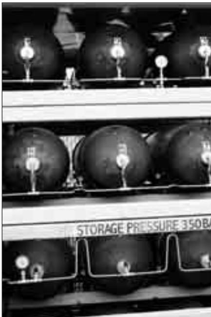
CLOCKWISE FROM TOP LEFT: BC Hydro's Ford Focus fuel cell vehicle (one of five in the Vancouver Fuel Cell Vehicle Program) beside the Hydrogen Highway station at Powertech Labs (Surrey). A close up of the fuelling receptacle on a hydrogen fuel cell powered Ford Focus. This is similar to natural gas vehicles. Carbon fiber and aluminum cylinders, made by Dynetek, safely store compressed hydrogen for use at a filling station.
